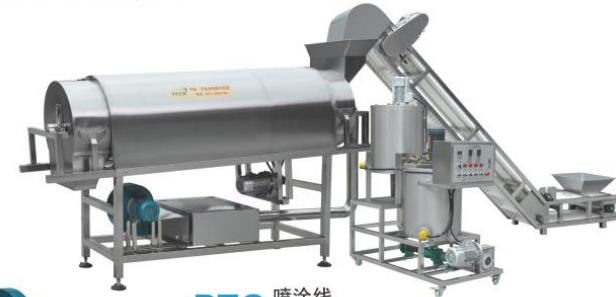
PTG 喷涂线 Coating Line
